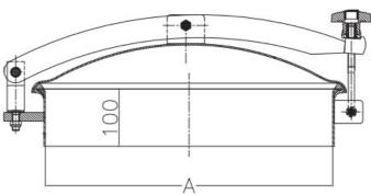
As you would expect from MSS, all pressureless manhole covers are coded with: *dimensions, type of material* and a *charge number*. So, it is completely recognisable and traceable (possibly by means of a certificate 3.1). Additionally, all seals comply with the FDA 177.2600 standard.
